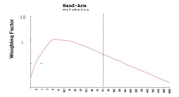
Because the vibration can occur on three axes, the measurement has to be done with this in mind. Historically, Lawrence said, in the UK all three axes were measured and control measures were set to manage the highest value. The new Directive (Physical Agents) (PAD) requires all three to measured and used to calculate the total, as follows: -
