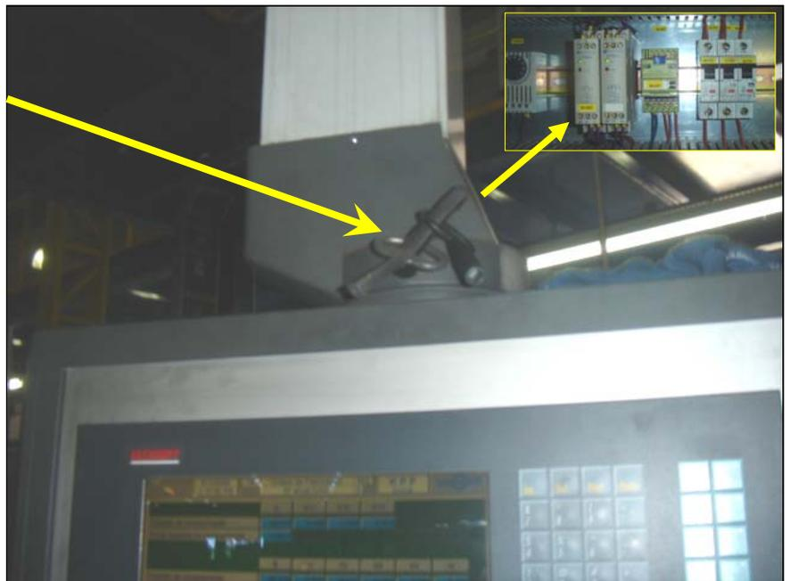
This operation is inherently unsafe and does not provide sufficient protection to a second party, out of site of the remote control panel.
