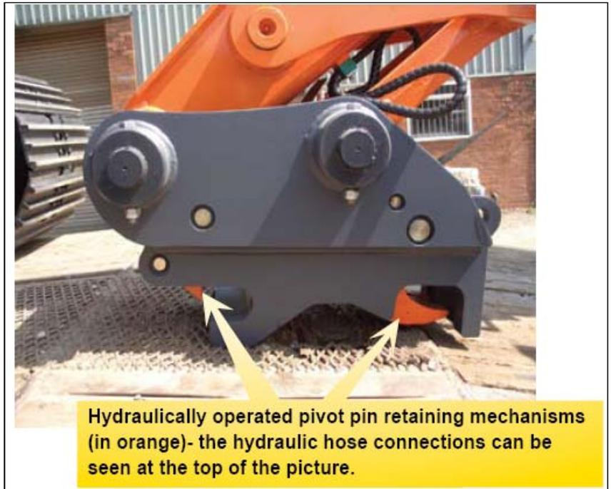
The problem may be partially overcome by an improved version of the device called a “Fully Automatic Quick Hitch”,
