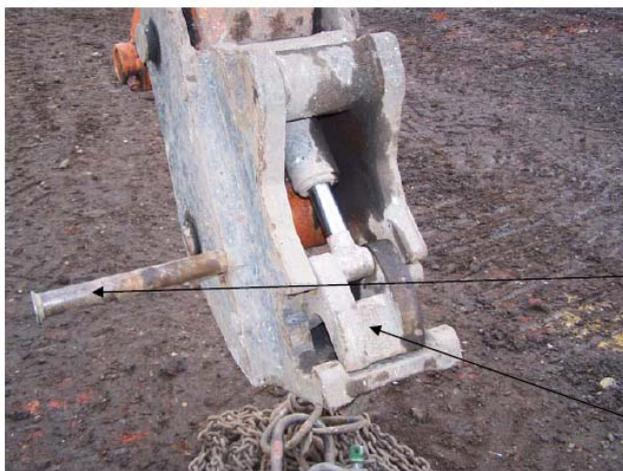
Photo 1: Semi-automatic type of QH (Safety pin about to be inserted)
