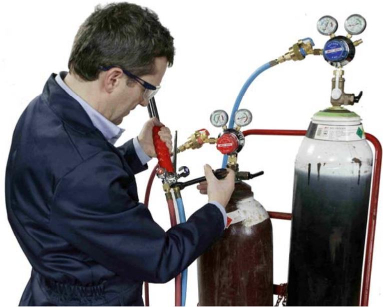
Colour-coded pipes on an Oxy-Acetylene rig
