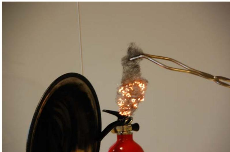
**Contact between battery and steel wool**
