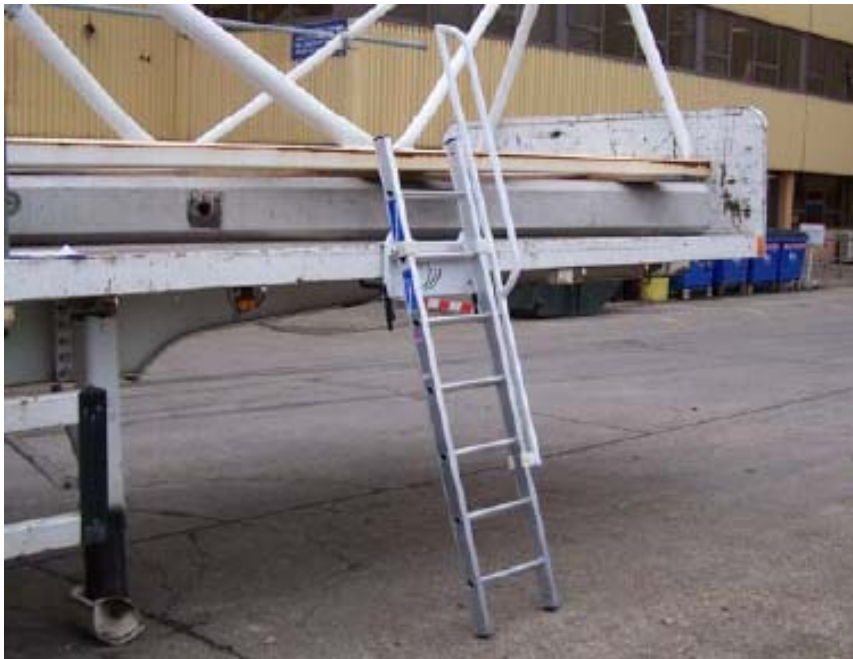
Improved ladder access with handhold to flatbed trailer
